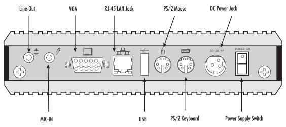
Figure 8. Ultra-Thin System rear connectors
